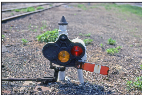
CO Tower controlled this dwarf signal on the siding of the former New York Central mainline between Cleveland and St. Louis.
